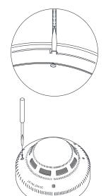
2) To remove the secured detector from its base, insert a small diameter screw driver into the large hole on the outer rim of the detector. Excessive force can damage the locking tab. While depressing the tab, rotate the detector counterclockwise.
