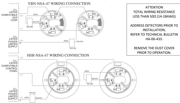
\* OPTIONAL WIRING CONFIGURATIONS FOR REMOTE ALARM INDICATOR LED, 9.6mA max output
